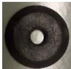
Figure 8: 5/16 concave rubber washer inserted between the fixed support and the hole in the lid of the container which is acting as a biodigester [19].
