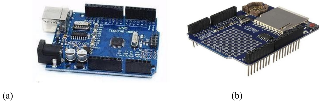
Figure 1: Arduino Uno Tenstar Robot Board (a) and DataLogger Module with integrated RTC (b).
