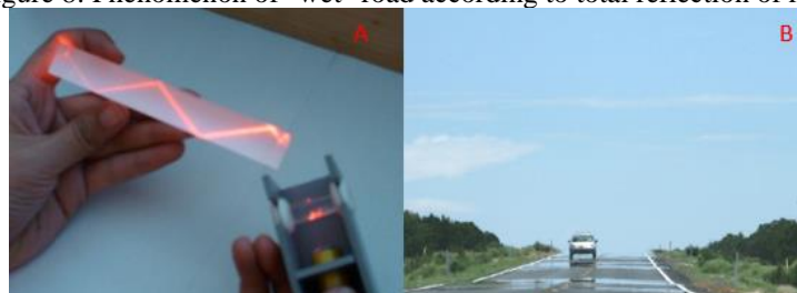
Figure 8: Phenomenon of "wet" road according to total reflection of rays
