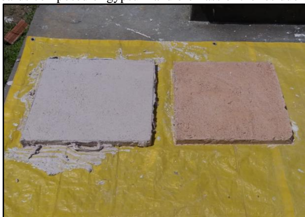
Figure 06 – Boards composed of gypsum and biomass of the residue of the açai seed
