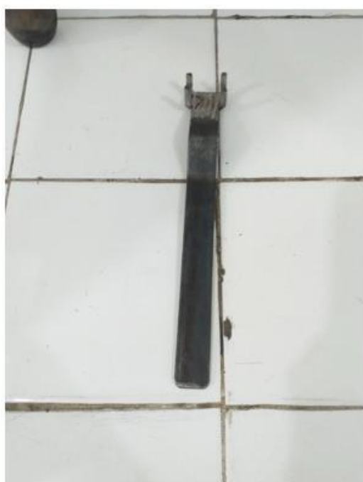
Figure 4 - Lever to be adapted to the gas outlet tap, so that the student had autonomy in relation to the opening and closing of the gas.
