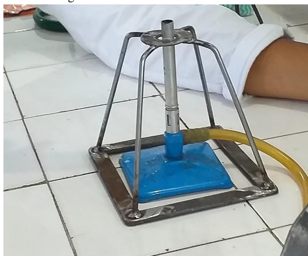
Figure 2 - Iron holder for Bunsen nozzle.
