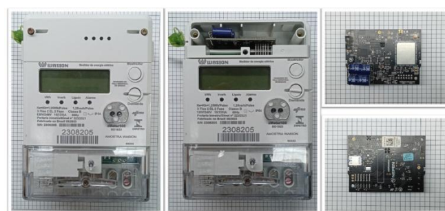
Figure 01: Wasion meters: On the left is the complete meter, in the centre is the top of the STM32WBA microcontroller, on the top right is the front of the microcontroller and on the bottom right is the back side microcontroller.
