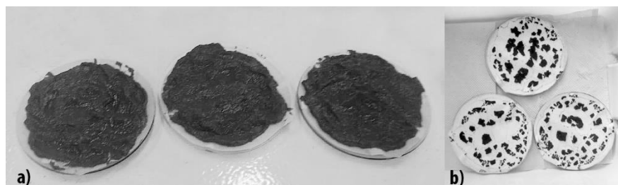
Figure 5: Biomass (PCBP) contaminated with Cr 6+ ion after the adsorption process. (a) Biomass on common filter papers arranged in an exhaust chapel for drying at room temperature; (b) Biomass on filter papers after 24 hours of drying in an exhaust chapel at room temperature.
