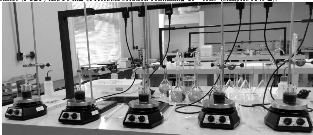
Figure 3. System used for adsorption of \text{Cr}^{6+} ions in heating plates with magnetic agitation and mixing in beakers of 100 mL, containing 2g biomass (PCBP) and 50 mL of residual solution containing \text{Cr}^{6+} ions (samples A to E).
