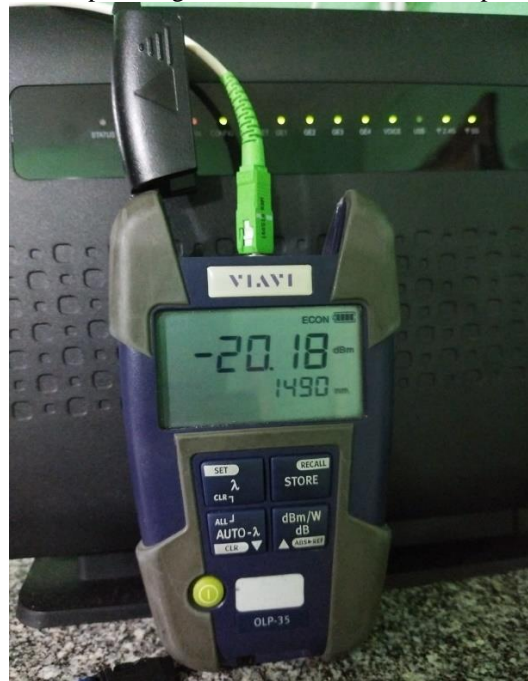
Figure 18- Optical signal measured on the ONT optical bead
