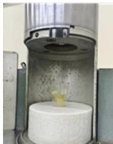
Figure 3. Samples on the Co-60 irradiator - GamaCell 220.
