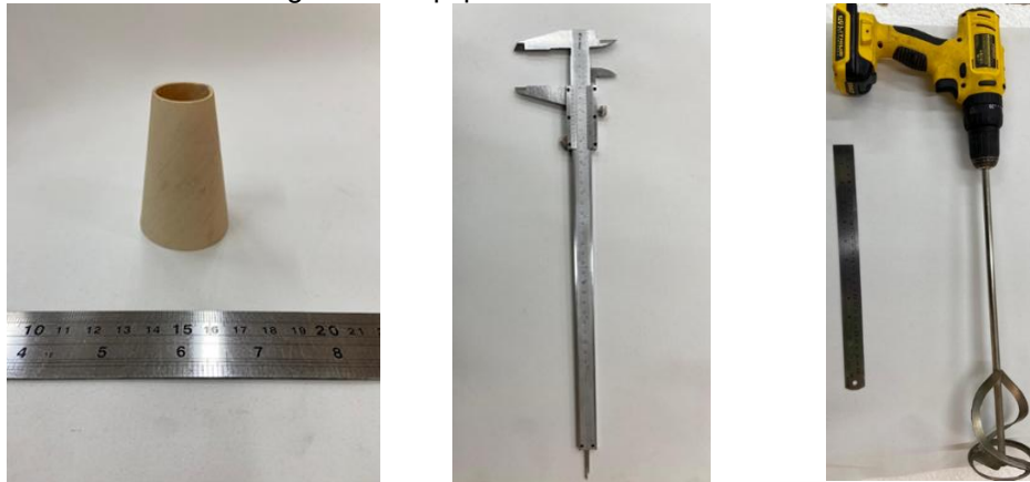
PVC conical trunk mold Analog caliper Drill with helical shank Source: Authors, 2025
