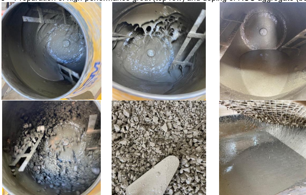
Figure 10 – Preparation of high-performance grout (top row) and doping of RCC aggregate (bottom row).
