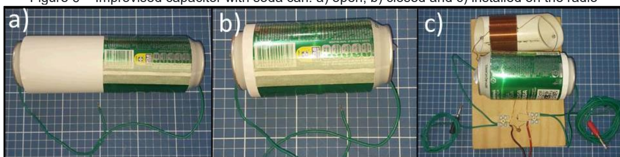
Figure 6 – Improved capacitor with soda can: a) open, b) closed and c) installed on the radio
