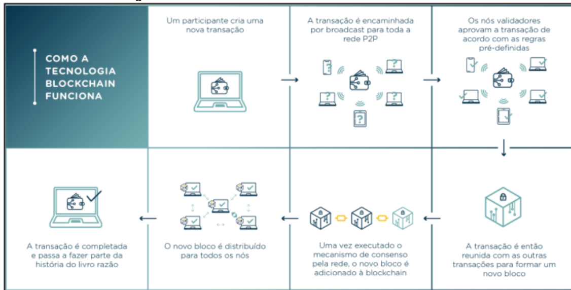
Figure 01 - Demonstration of how the blockchain works
