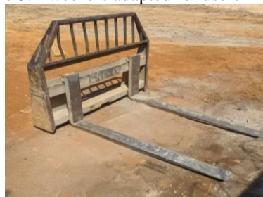
Figure 3. Tweezers adapted for use on Bobcat
