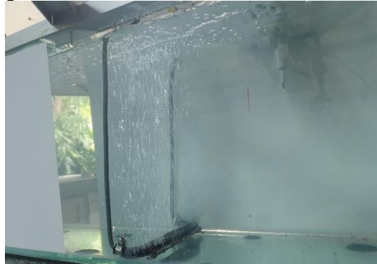
Figure 2 – Image of the curtain formation test in the bubble curtain system.
