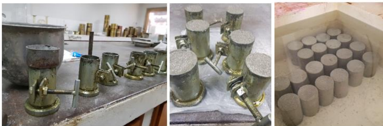
Figure 1 - Molding and submerged curing of specimens in mortar
