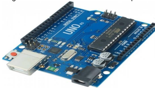
Figure 11 - Arduino Uno used in data acquisition
