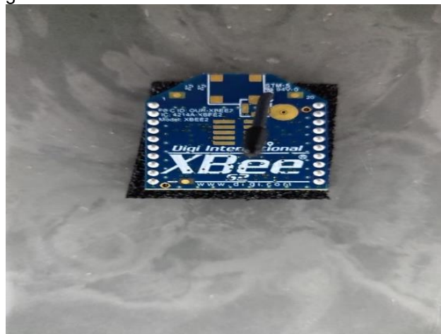
Figure 12 - Xbee communication module used in Arduino
