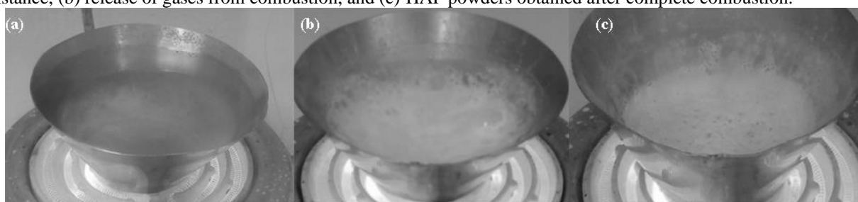
Figure 3 – Stages of obtaining HAP by combustion reaction, using urea as fuel. (a) Heating of the reactant mixture at the resistance, (b) release of gases from combustion, and (c) HAP powders obtained after complete combustion.
