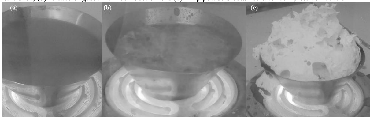
Figure 2 – Stages of obtaining HAP by combustion reaction, using glycine as fuel. (a) Heating of the reactant mixture in the resistance, (b) release of gases from combustion and (c) HAp powders obtained after complete combustion.
