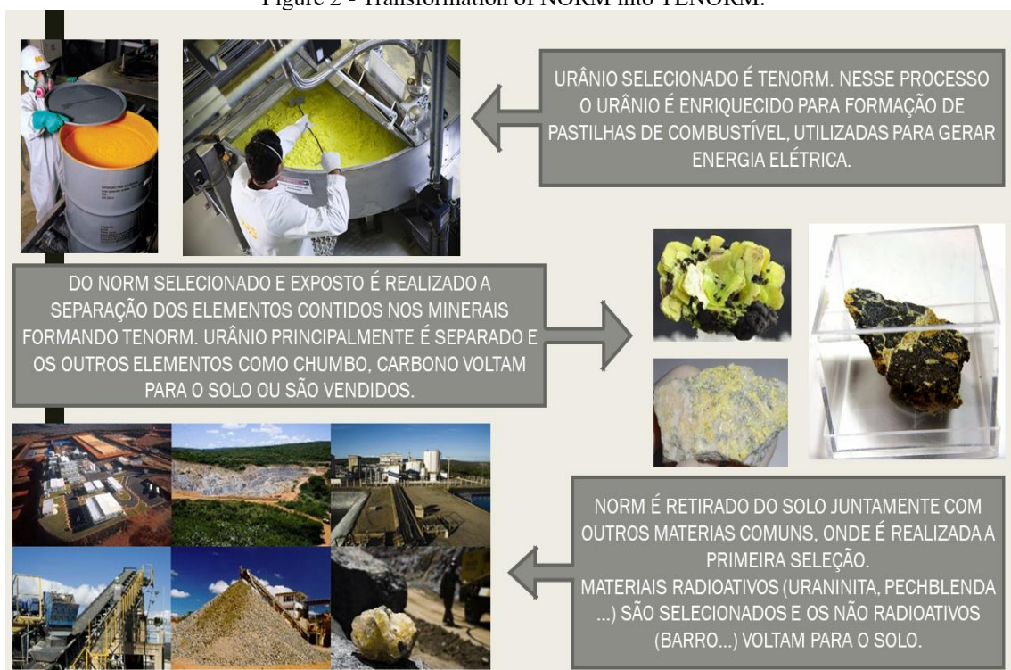
Figure 2 - Transformation of NORM into TENORM.
