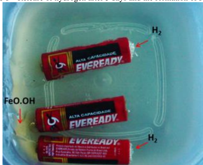
Figure 8 – Release of hydrogen after 5 days and the formation of FeO.OH
