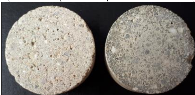
Figure 16 – Surface aspects of concrete specimens after 600 hours of testing
