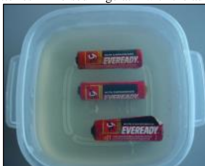
Figure 7 – Used batteries immersed in gelatin with the addition of 3.5% NaCl
