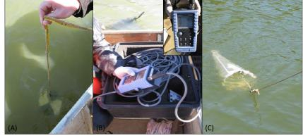
Figure 2 – Equipment used to monitor water quality. (A) Secchi disc; (B) multi-parameter probe; (C) Plankton network
