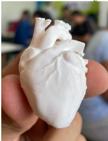
Figure 6 – Human heart manufactured using a 3D printer
