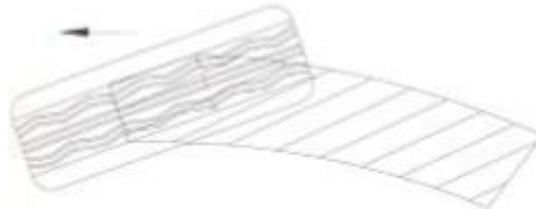
Figure 2: Skidding under acceleration
