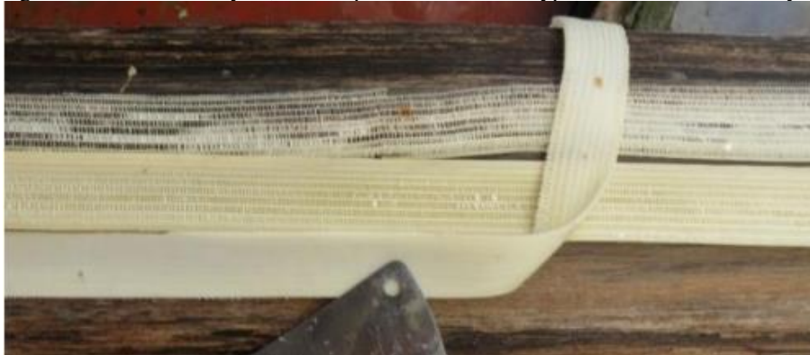
Figure 1. Pseudostem layers, from top to bottom: mesh type, hard fiber and soft layer.
