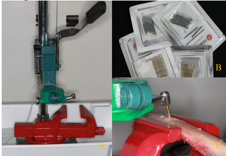
Figure 2: A- Contra angle attached to the verticalizer; B- Steel and DLC drills; C- Drilling length 7.0mm.
