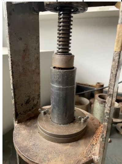
Figure 2.9 – Manual compaction process of specimens.
