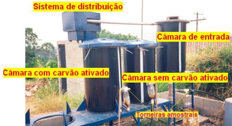
Figure 1 – FEAGRI/UNICAMP Slow Filtration System.
