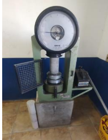
Figure 14 – Samples in the Hydraulic Press.
