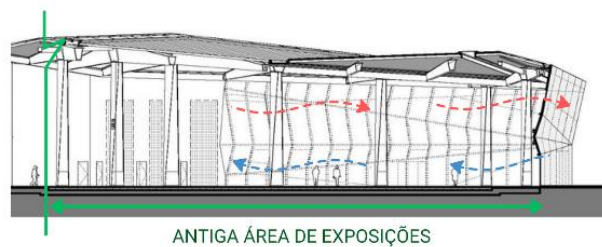
Figure 16. Cross Ventilation Scheme
