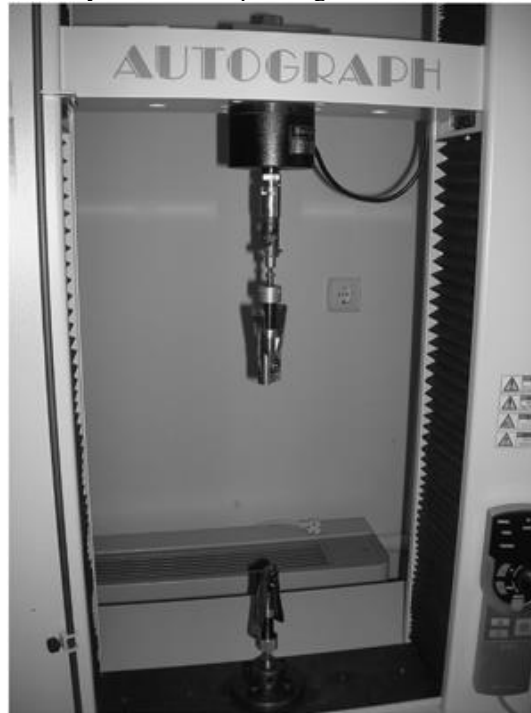
Figure 6. Dynamometer operating a breakdown stress test.
