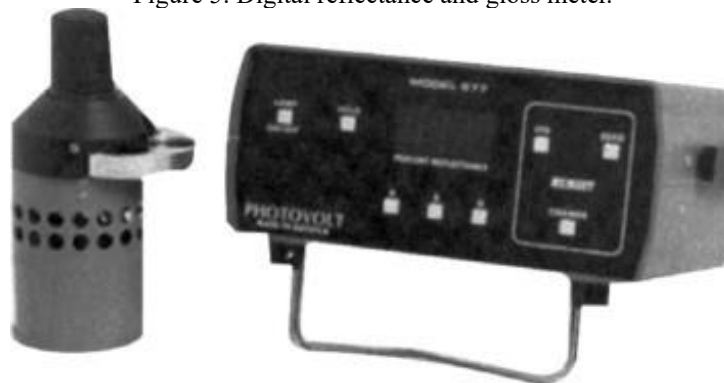
Figure 5. Digital reflectance and gloss meter.
