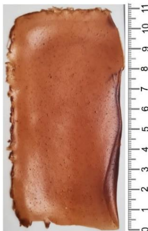
Figure 1 - Photographic record of the starch-based polymer blend obtained from the mesocarp of O. phalerata . Scale in cm.
