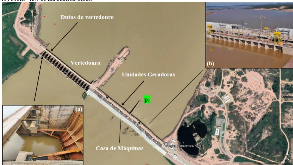
Figure 1 – Structure of the study areas of the Jirau HPP (Source: Google Earth) with emphasis on (a) View span 18 of the spillway, with a closed gate upstream, preventing the flow of water through the downstream opening (Source: Authors), and (b) Front view of the suction pipes.
