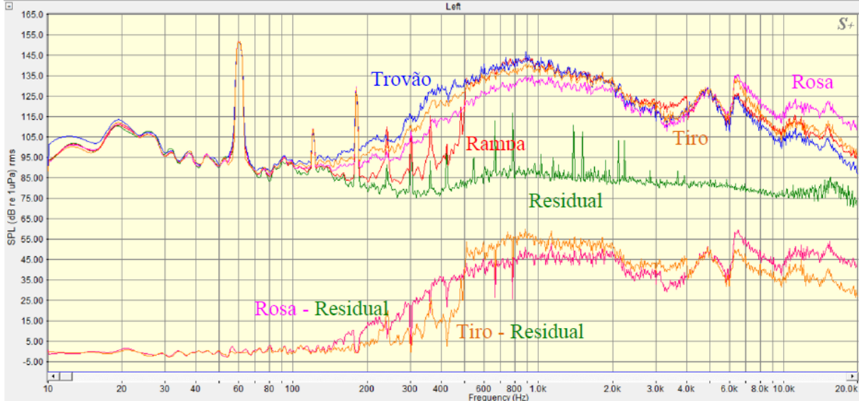
Figure 6 – Spectrum of environmental noise in the spillway when the acoustic source reproduces each of the pre-defined noises (with sonar turned off): Pink noise (pink), Ramp noise (red), Thunder noise (blue) and Gunshot noise (orange).
