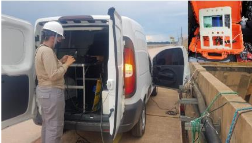
Figure 4 – Acoustic and ichthyofauna monitoring system implemented in the spillway of the Jirau HPP.
