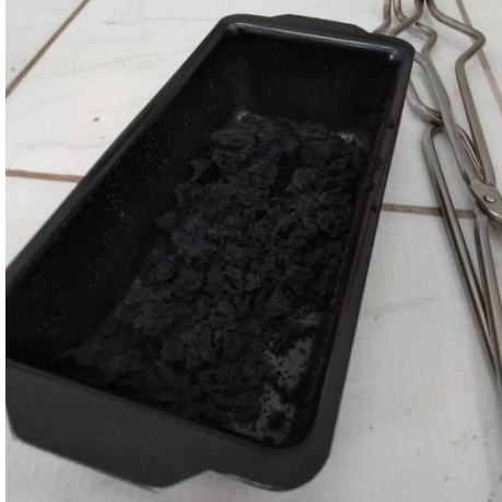
Figure 5 - Result of copper pre-firing.
