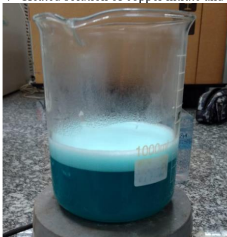
Figure 4 - Heated solution of copper nitrate and gelatin.
