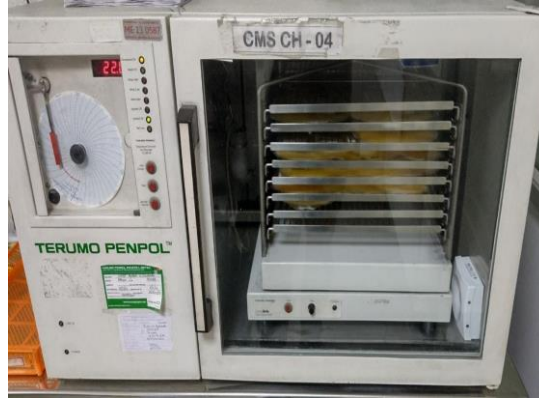
Fig 7. IoT device in Platelet Agitator & Incubator
