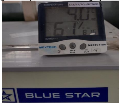
Fig 4. Data logger: Temperature Monitoring System for Refrigerator
