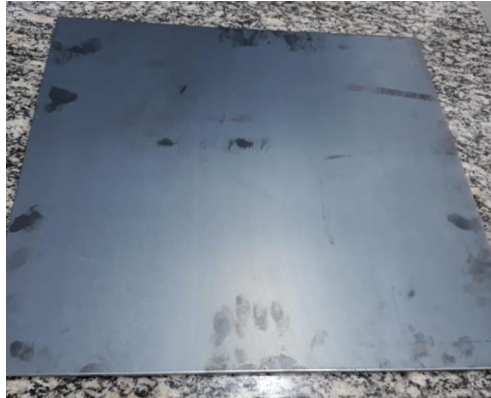
Figure 1 – 1020 Steel Plate used in this research, as received. Source: The author, 2023
