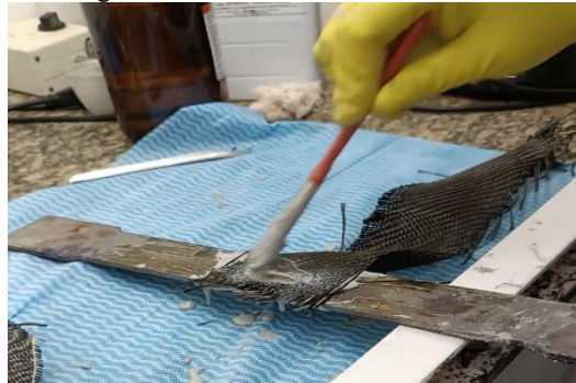
Figure 7- Application of the adhesive together with the carbon fiber on the other layers. Source: The author, 2023.
