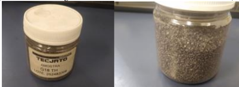
Figure 2 – Shot blasting G18 TH and Lot: 262483208. Source: The author, 2023.
