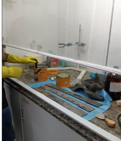
Figure 4 - Handling of the adhesive was carried out inside the fume hood. Source: The author, 2023
