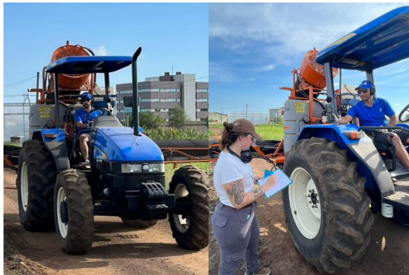
Figure 1 – Measurement of noise levels emitted by a tractor-sprayer mechanized assembly at the agricultural tractor operating station
