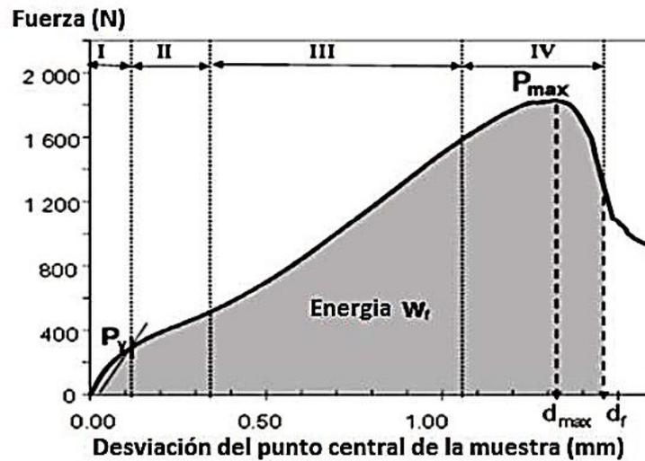
Fig 3 illustrates the force-displacement curve obtained by SPT, in this curve four different zones can be distinguished: zone I elastic deformation, in this zone a slight influence is observed at the initial contact of the punch with the specimen, zone II elastoplastic transition, in some parts of this zone specifically those that are in contact with the periphery of the punch, Zone III is the result of generalized plastic deformation, zone IV characterized by plastic instability and fracture.
