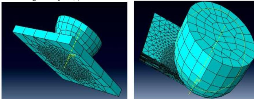
In FEM, the accuracy of the method depends on several factors present in the mesh, such as the number of nodes, type, size, and number of elements. The solution tends to converge to the exact solution as the mesh is refined (examples in Figure 4), i.e., the greater the number of elements, the greater the accuracy of the results.
