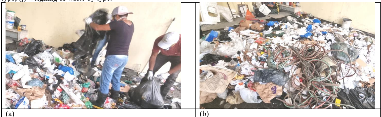
Figure 4. Gravimetry: (a) Removal of waste from plastic bags; (b) mixing of waste; (c) quartering; (d) separation of 1m 3 of waste; (e) and (f) weighing of mixed waste; (g) and (h) weighing of waste separated by type; (i) separation of waste by type; (j) weighing of waste by type.
