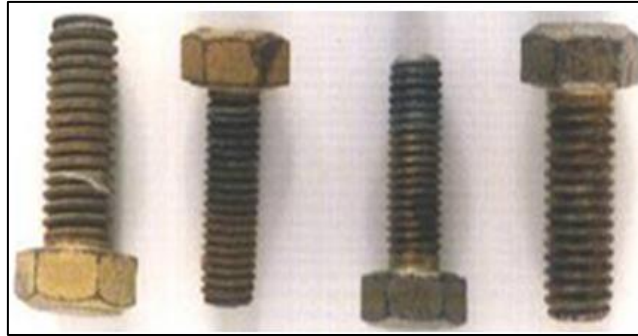
Figure 6 - H 2 S attack on cadmiated screws from 150 to 200°C
