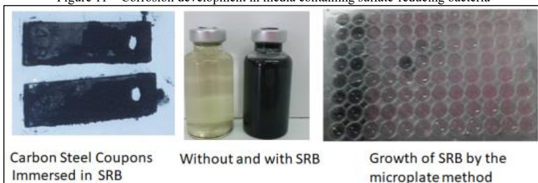
Figure 11 – Corrosion development in media containing sulfate-reducing bacteria
