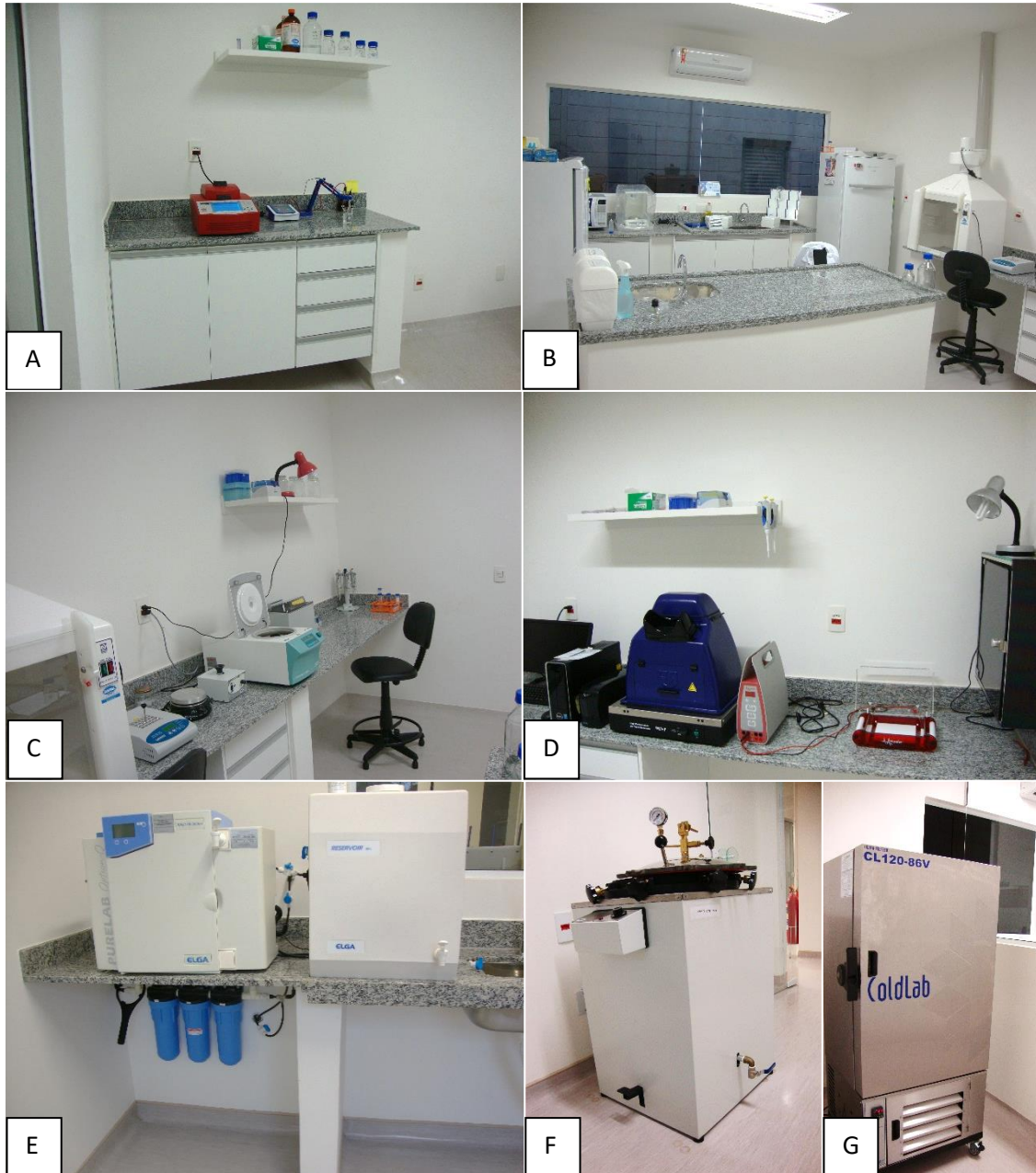
Figure 3. Molecular Biology Laboratory, including electrophoresis room. A - Bench with thermocycler and pH meter. B - Workbench with equipment and sinks. C - Workbench where reactions are prepared, with equipment and micropipettes. D - Electrophoresis room with tank and photodocumentator. E - Ultrapure water room with respective equipment. F and G - Autoclave and ultrafreezer (-80°C).
