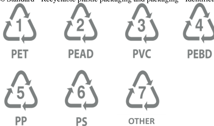
Figure 3. ABNT NBR 13.230 standard with the symbology of identification of plastic products and raw materials. [Image source: ABNT NBR 13230 Standard - Recyclable plastic packaging and packaging - Identification and symbology].
