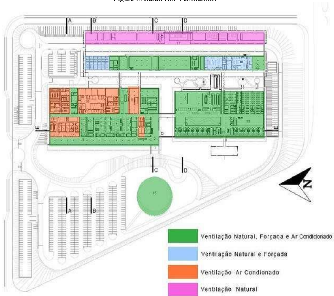
Figure 8: Sarah Rio Ventilations
