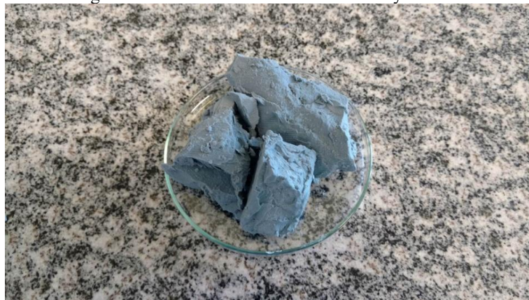
Figure 1- Chromium residue from a tannery WWTP.
