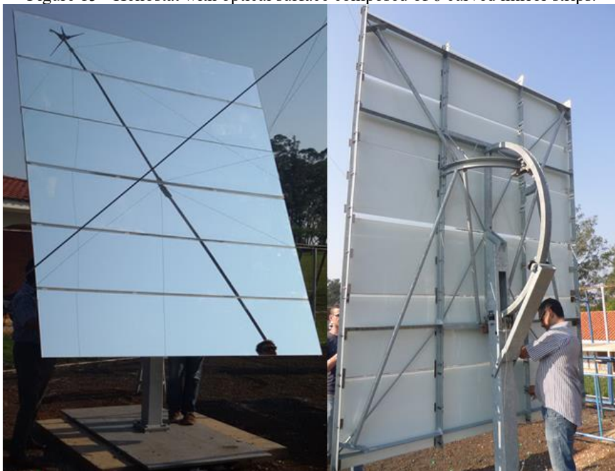
Figure 15 - Heliostat with optical surface composed of 6 curved mirror strips.
