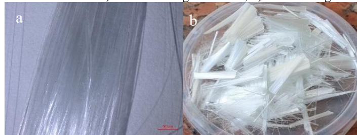
Figure 2. Glass fibers: a) before cutting to 15 mm, b) after cutting to 15 mm.
