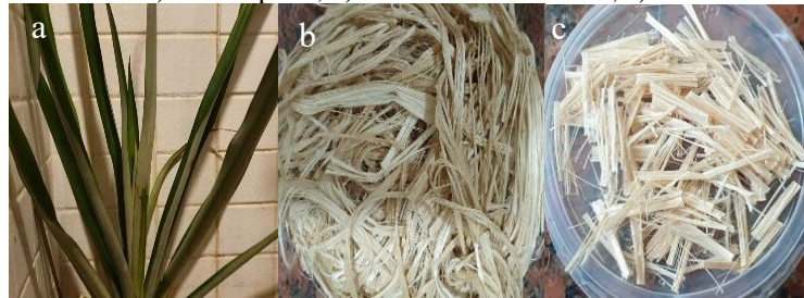
Figure 1. Curauá fiber: a) curauá plant, b) curauá fiber in natura, c) curauá fiber with 15 mm.
