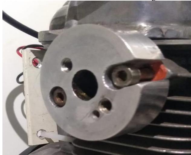
FIGURE 8. Exhaust manifold 1E machined and fixed to the engine. Source: Authors (2022).
