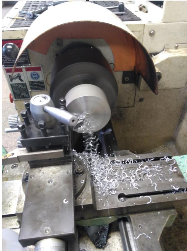
FIGURE 3. Mechanical Lathe turning aluminum billet. Source: Authors (2022).
