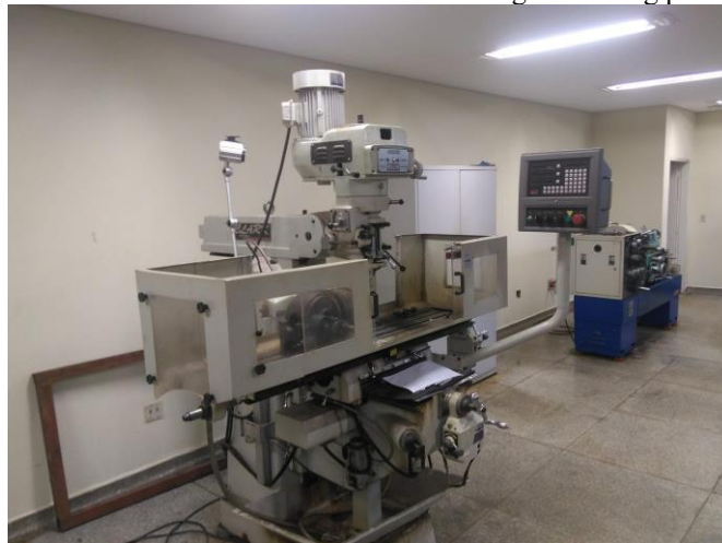
FIGURE 4. Milling machine combined with CLARK MACHINE digital reading panel. Source: Authors (2022).
