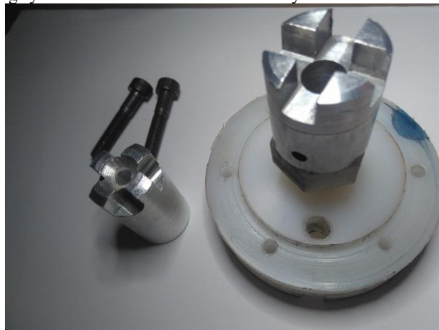
FIGURE 9. Machining system machined in aluminum and nylon with screws. Source: Authors (2022).
