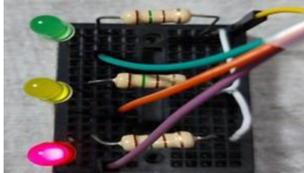
Figure 9. LEDs used in the prototype to simulate complementary signaling to the maintenance team
