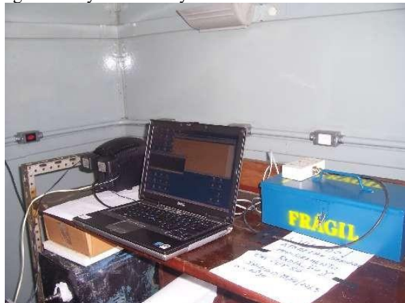
Figure 3 – Compact gamma-ray detection system. The scintillator is inside the blue metal case.
