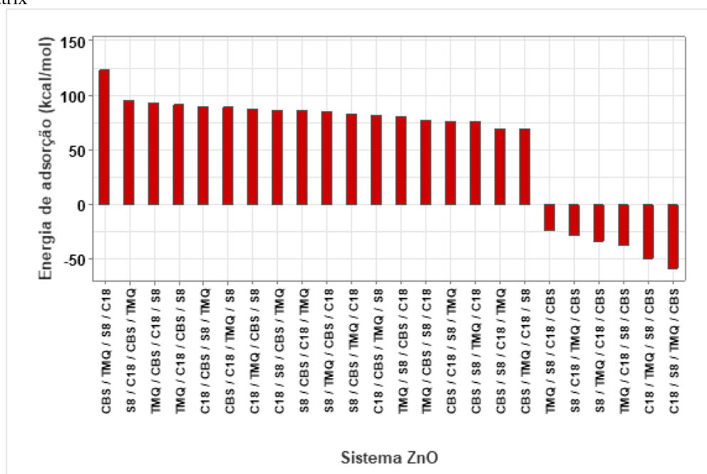
Figure 6: Values of the adsorption energy for the ZnO system, according to the order of addition of the different additives to the NR matrix
