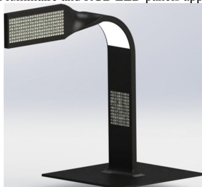
Figure 3 – Initial idea of the traffic light with luminaire and RGB LED panels applied to intelligent traffic management.
