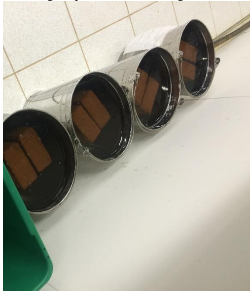
Figure 08 - submerged specimens after being removed from the oven
