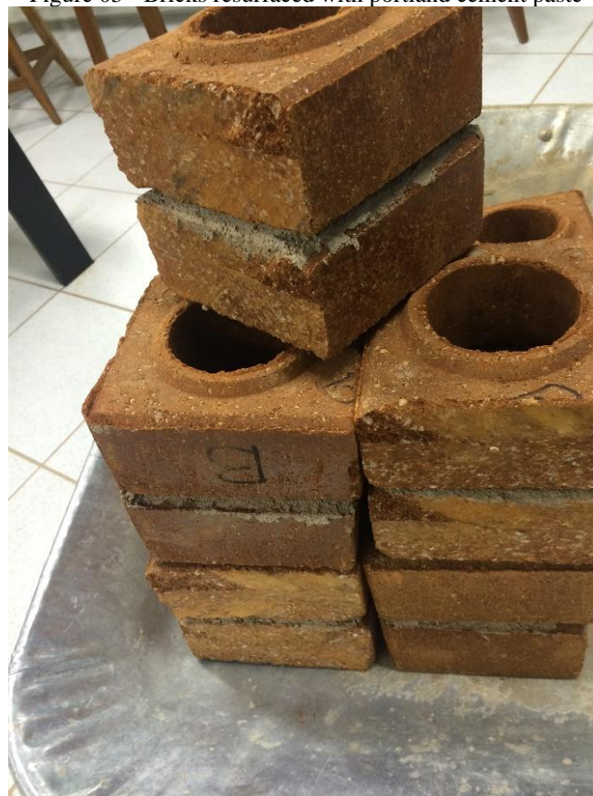
Figure 03 - Bricks resurfaced with portland cement paste
